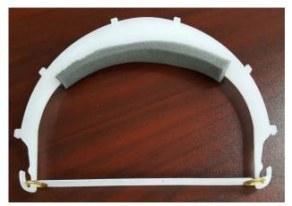
**Visor:** The visor is made from .220 white cast acrylic. Our design keeps the shield at an appropriate distance to reduce fogging. The tabs on the front are designed to make the shield snap on and off easily. There is a foam strip where it rests against the forehead to assist with comfort in long term use. An elastic band easily attaches to the frame. Elastic band is included.
